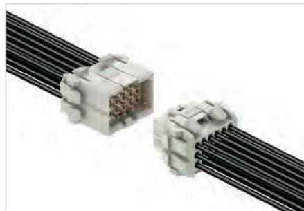
Rectangular plug-in connector for use with crimp contacts. Can be used as universal coupling, but also with the PCB variations. The crimp contacts guarantee a high connection density. The CS 1.6 or CB 1.6 contacts are used here. The connectors can be coded and locked together with their mates. Supplied in cardboard box.
