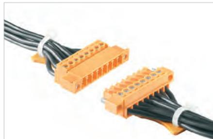
Female plug with screw connection and strain relief for the connected wire. Wire outlet 180° (wire is straight on to the direction of plugging).
