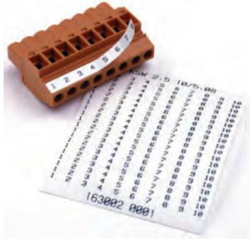
KSW marking strips are suitable for labelling multi-pole PCB terminals and connectors. The white, self-adhesive strips are made from a non-PVC, environmentally friendly material. These marking strips provide individual printing, i.e. are suitable for every pitch. Available in two widths: 2.5 and 4.0 mm.
