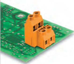
Double-level PCB terminal with our proven clamping yoke screw connection in 9.52 mm pitch, suitable for wire cross-sections up to 6 mm<sup>2</sup>.
