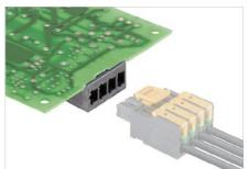
Modular male headers in 5.00 mm pitch with 270°  $\,$ outgoing elbow made of high performance material PA9T, which can be used for both reflow and wave soldering process.
