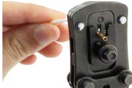
7) Tighten sharply the handles to the end of the mechanism
