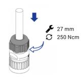
Screw the cable gland to the connector body.
