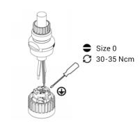
Unscrew the PE-contact, insert the PE-conductor and tighten again.
