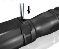
• Then push on the screwdriver and pull slightly on the plug do disconnect it
