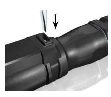
• To disconnect the plug, when Protective Shroud is used, please use a screw driver and put the screw driver into the hole of the protective shroud
