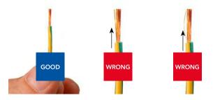
6) Position the contact in the bottom of the tool by checking its orientation. Maintain the wire in position.
