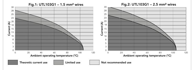
The rated current is defined as uninterrupted continuous current that a connector can take when all contacts are energized simultaneously without exceeding the maximum limit of temperature. The ground contact is never loaded.
